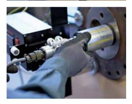
Measurement directly on the extruder line. Measurement range of the sensors: 47 - 133 mm in diameter.
