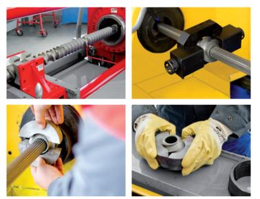
Clamping the shaft with screw elements into the FD dismantling machine, installation of the aluminium shells before the dismantling process, removal of the dismantled screw elements, finished and new assembly.
