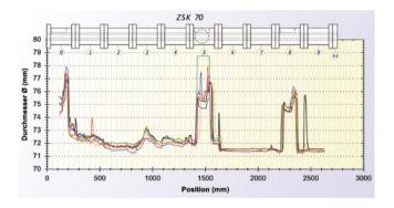
Example of measuring result ZSK 70, diameter 71.3 mm
